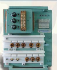
resonant converter based high voltage power supplies with integral floating-deck modulator for TWT amplifiers & Microwave Power Modules. These rugged power supplies are highly efficient, reliable, and protected against overload and short circuits. High frequency resonant converters are very compact, have low output ripple and very low arc dump energy. Stabilized feedback loop ensures highly stable helix voltage.
